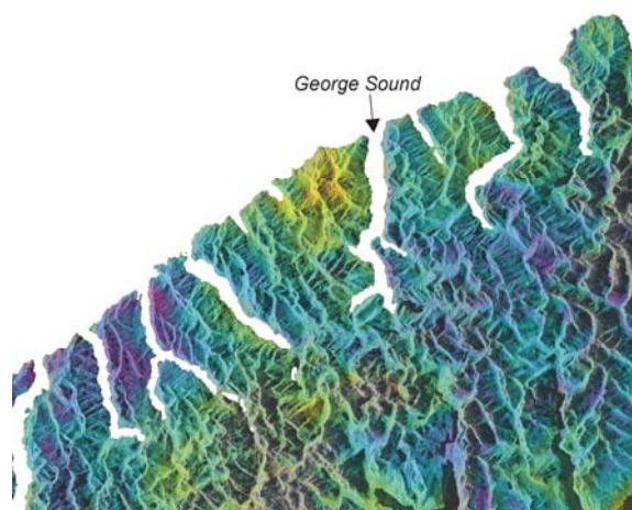
Figure 6: Wrapped differential interferogram calculated from ALOS PALSAR images acquired on 22-Oct and 22-Jan. A post seismic signal is observed around the coast west of George Sound with a maximum LOS value around 5 cm.
