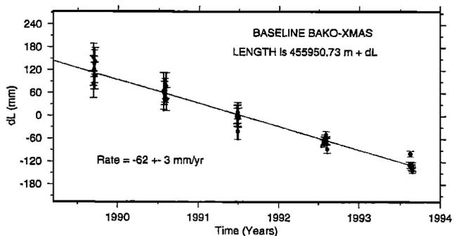
**Figure 4.** Daily estimates of the distance between XMAS and BAKO from the Kalman filter back solution. Formal one sigma error bars are shown. Weighted least squares line of best fit yields a rate of change of distance of  $-62 \pm 3$  mm/yr.
